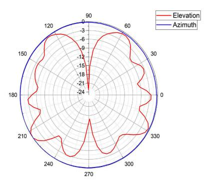
Frequency: 5.15GHz Max Gain: 3dBi
